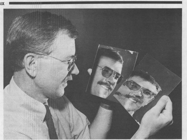
DICK PETTIT (now 7243) holds two versions of acrylic reflective films made by 3-M. Despite its unacceptable light-scattering tendency, the original 1974 version (right) appealed to Dick for use on early solar parabolic troughs. Following a Sandia/3-M collaboration, the company came up with a new film (left) that could be used on troughs, while Dick developed equipment to precisely characterize performance of reflective films.
